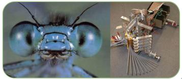
Morphological computation. Facet distribution of insect eye and robot system 'Eyebot' with an artificial compound eye, which can autonomously modify the angular positions of the individual
