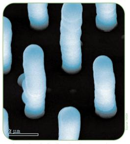
Array of vertically aligned carbon nanotubes grown using plasma enhanced chemical vapor deposition is intercalated with SiO<sub>2</sub> to provide a bottom-up process for developing interconnects. These vertical interconnects are ideal for DRAM applications and threedimensional architectures.
