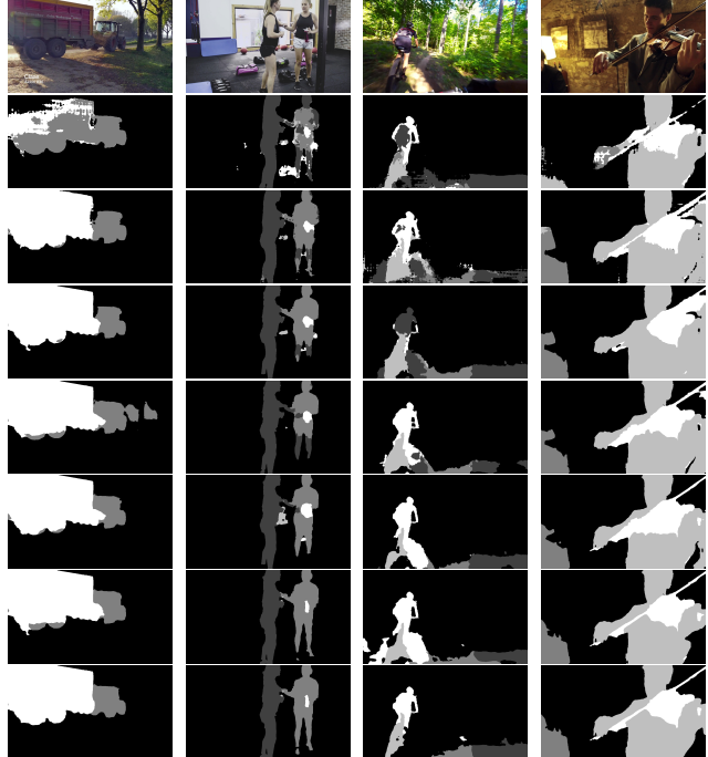
Figure 4: The impact of successive interactions on the quality of the segmentation outputs. The top row illustrates the input images and the segmentation results for consecutive interactions are depicted in the 2nd to 8th rows.
